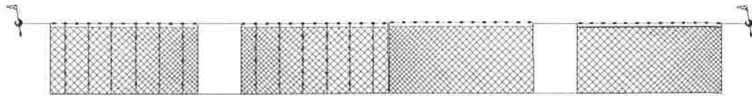
Figure 1 Configuration of experimental gill-net, total length = 240 m 4 off panels (each 55 m long by 18 m deep) 2 Modified panels with reflectors + 2 Unmodified + 2 gaps (10 m wide).
